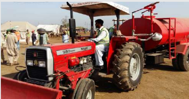
» Water Bowser being readied for a sprinkling operation
